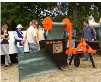
Michael Boeree from Omaru Engineering-traveled from Sydney to show the audience how easy it is to install silt fence with the Silt Fence Plow.
