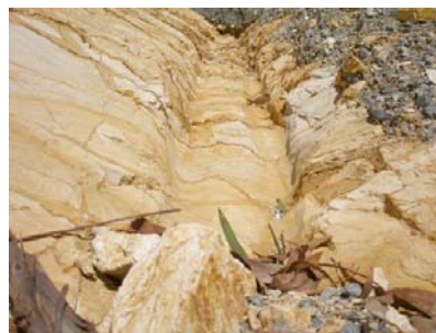
Dispersive nature of a parent material which also has a pH of 3.5 making landscaping options limited.
