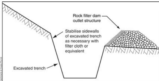
**Figure 1 – Sediment trench with rock filter dam outlet structure**
