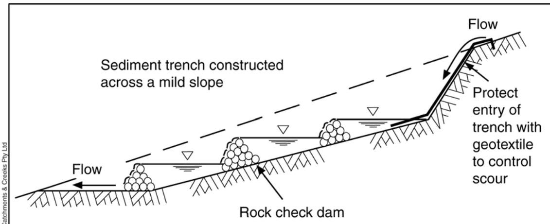
**Figure 5 – Long-section of a sediment trench excavated diagonal to a slope**
