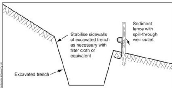
**Figure 3 – Sediment trench with sediment fence outlet structure**
