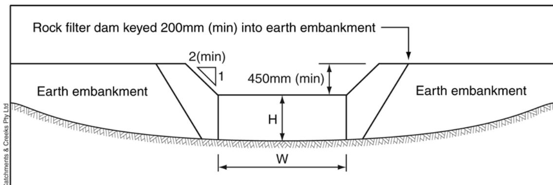
**Figure 11 – Rock filter dam integrated into fill embankments**
