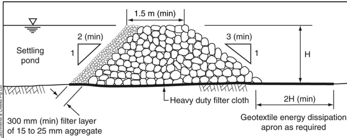
**Figure 6 – Rock filter dam outlet system with aggregate filter**
