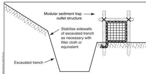
**Figure 4 – Sediment trench with modular system outlet structure**
