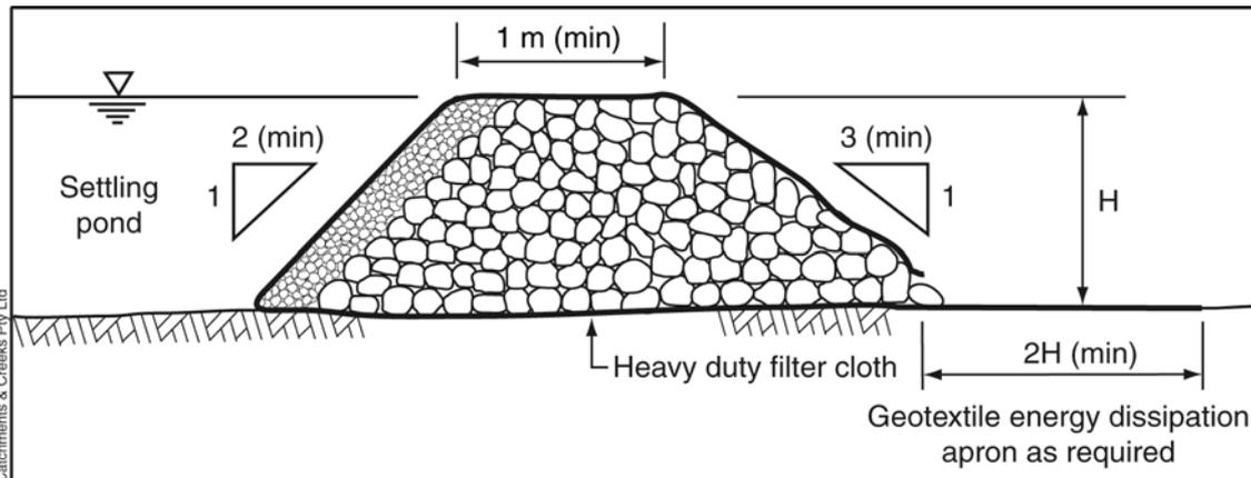
**Figure 7 – Rock filter dam outlet system with aggregate and geotextile filter**
