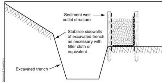
**Figure 2 – Sediment trench with sediment weir outlet structure**
