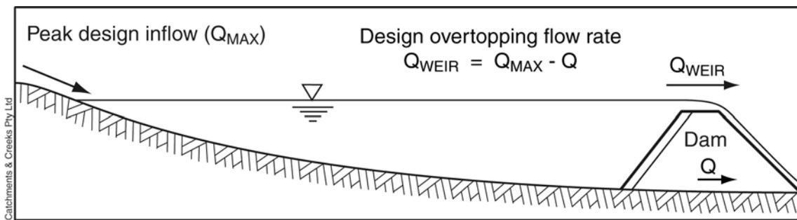
**Figure 10 – Maximum design flow condition**
