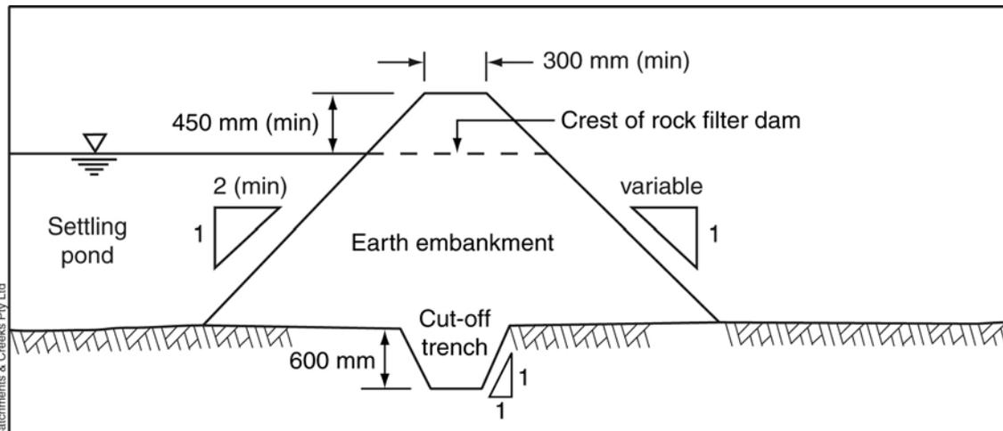
**Figure 8 – Typical dimensional requirements for constructed fill abutments**
