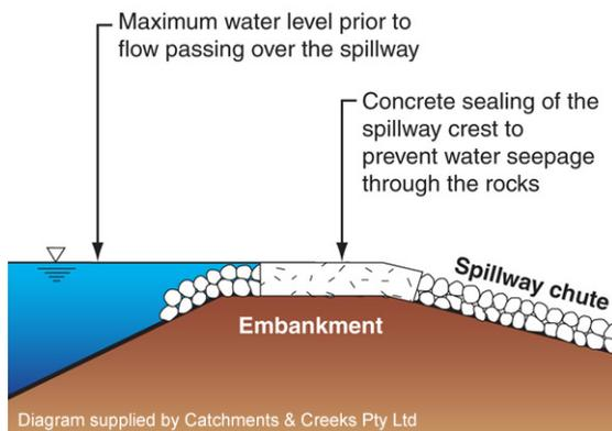
Figure 21 – Sealing of spillway crest
