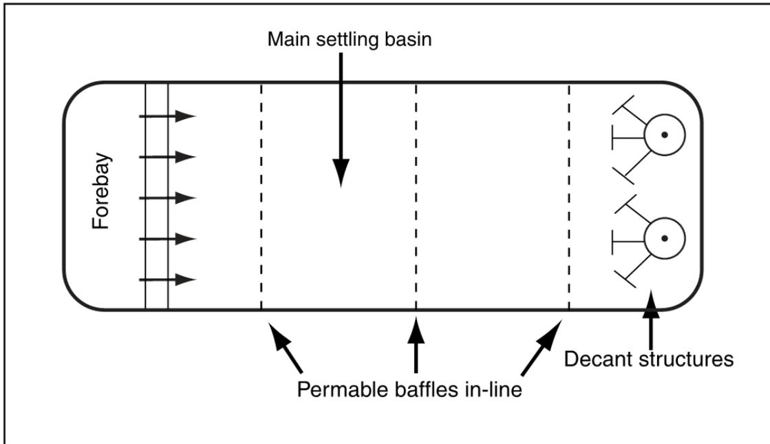
**Figure 7 – Typical arrangement of in-line permeable baffles**
