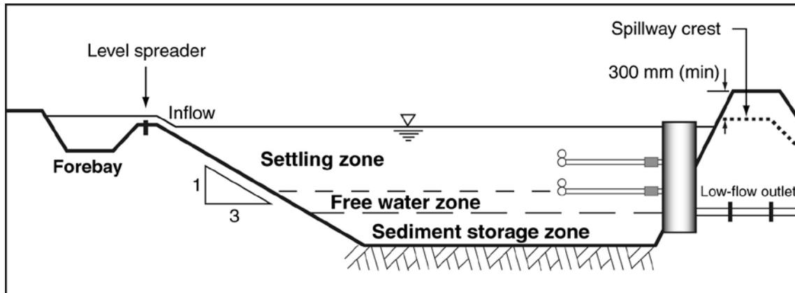
**Figure 1 – Long-section of a typical Type A basin**
