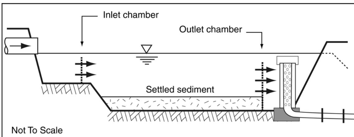
**Figure 8 – Typical arrangement of outlet chamber (long section)**
