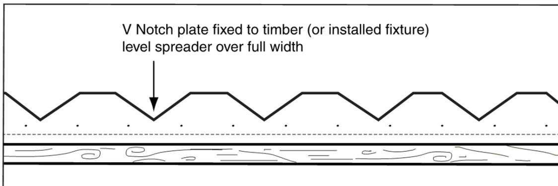
**Figure 13 – Typical detail for multiple V-notch weir plate**
