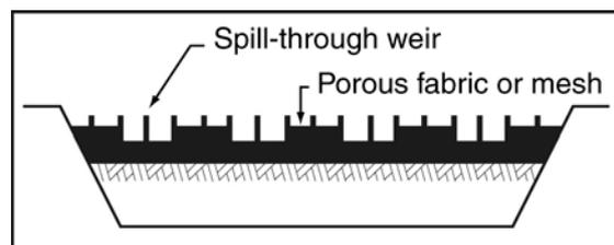
Figure 17(b) – Barrier with multiple spill-through weirs
