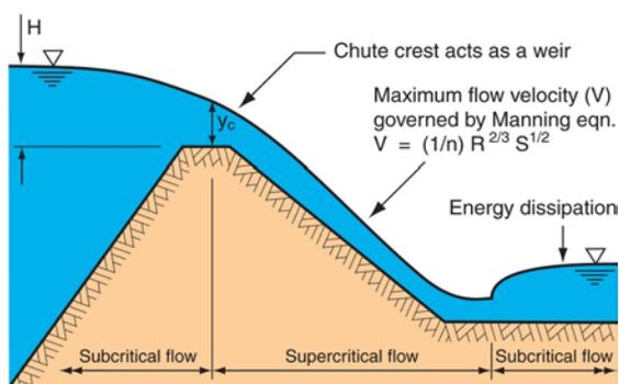
Figure 20 – Basin spillway hydraulics
