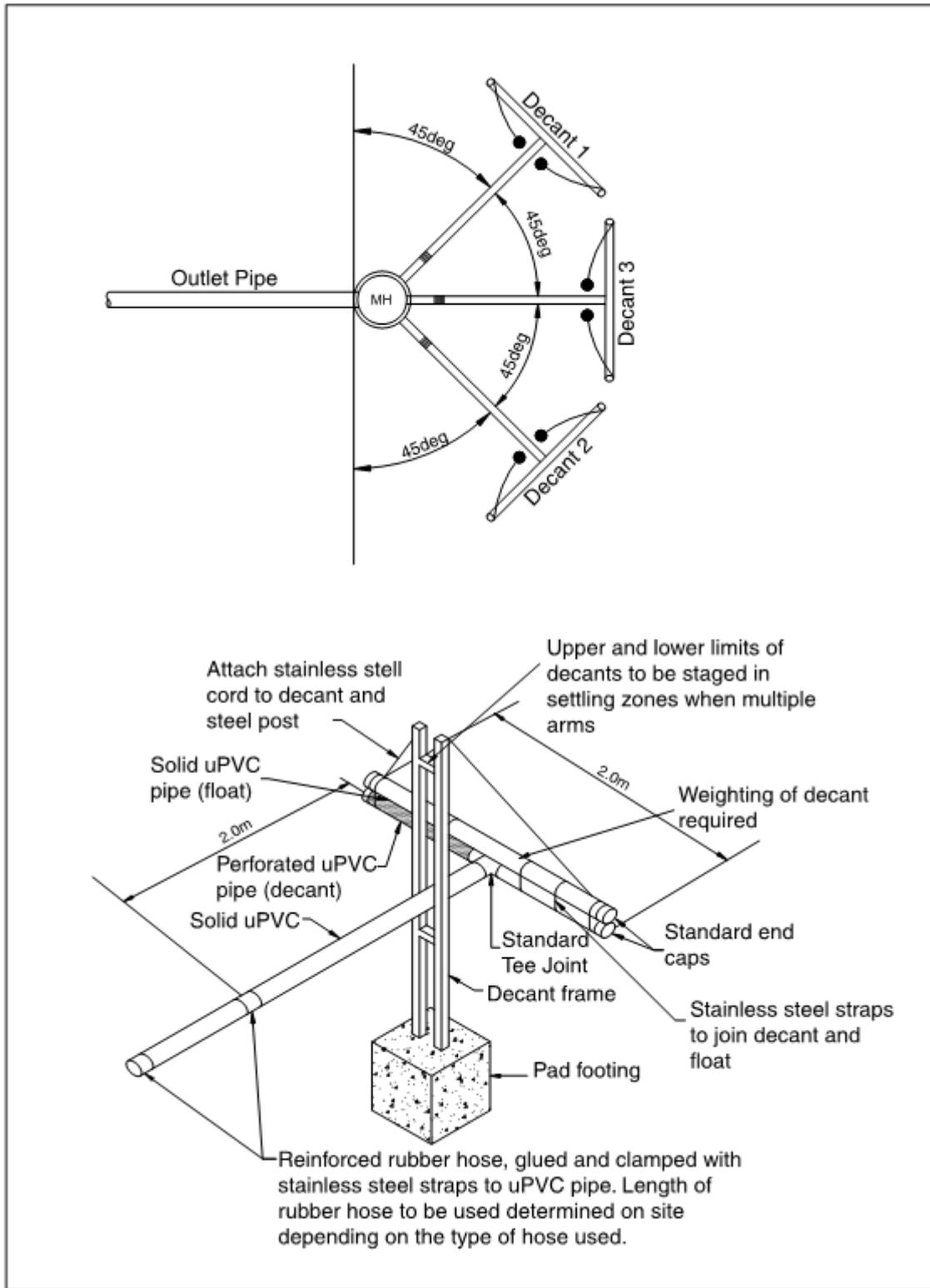
Figure 19 – Auckland-type floating decant system for Type A basins
