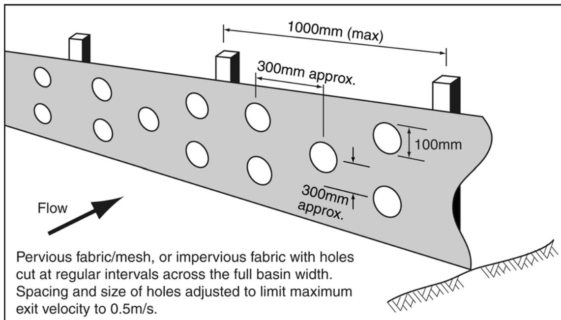
**Figure 18 – Example arrangement of perforated fabric inlet baffle**
