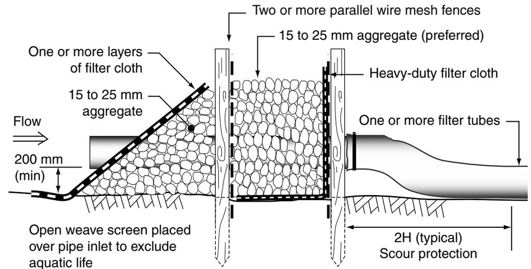
**(d) Sediment weir with filter tube**
