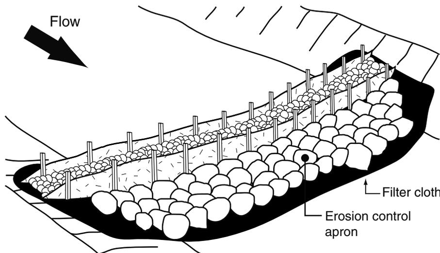
**(c) Sediment weir with downstream rock splash pad**
