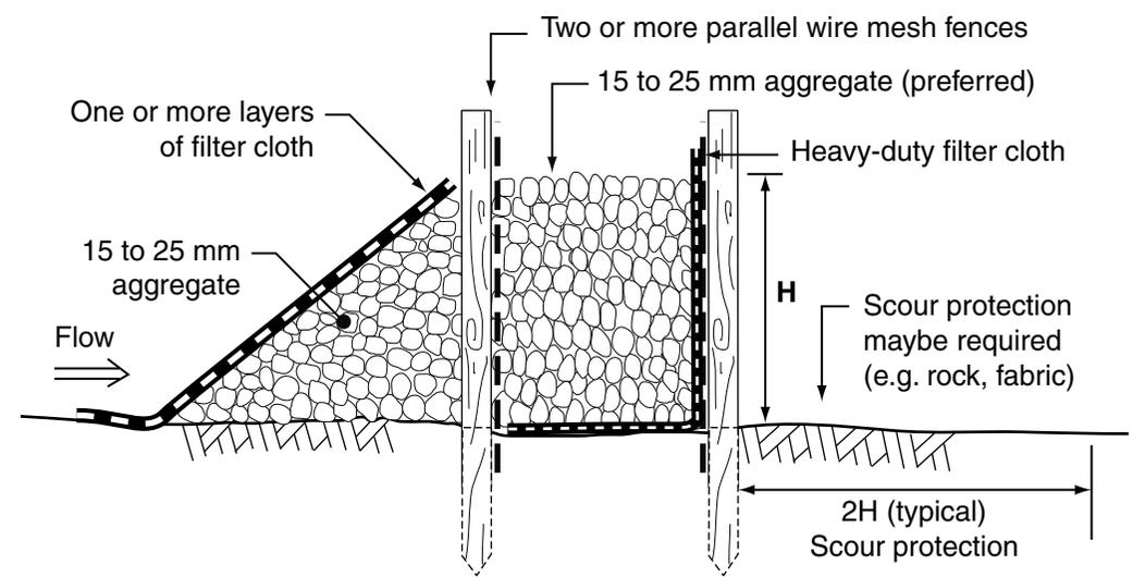
**(b) Sediment weir with aggregate and geotextile filter**
