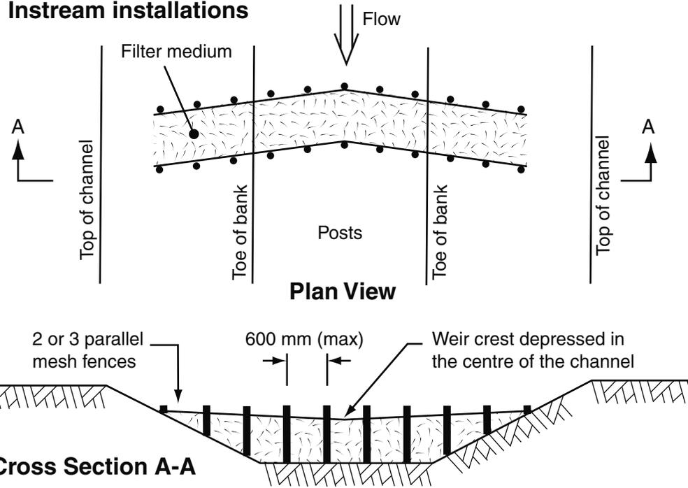
**(a) Typical installation of an instream sediment weir**
