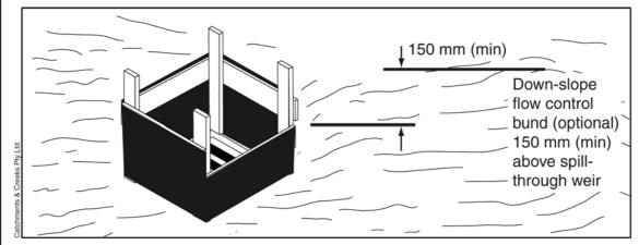
Figure 5 – Fabric drop inlet protection shown with an optional flow control bund to manage water ponding around the stormwater inlet
