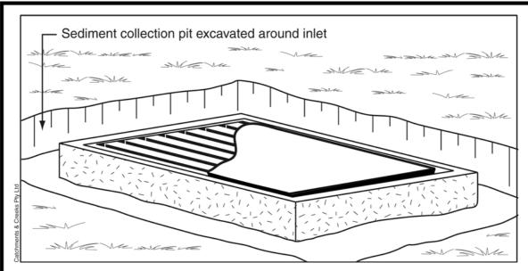
Figure 1 – Fabric wrap drop inlet protection (fabric shown partially exposed for visual display purposes only)
