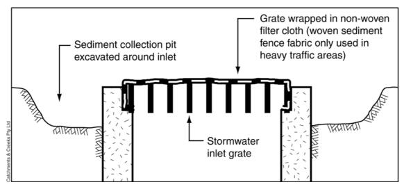
Figure 2 - Fabric wrap drop inlet protection with optional sediment collection trench
