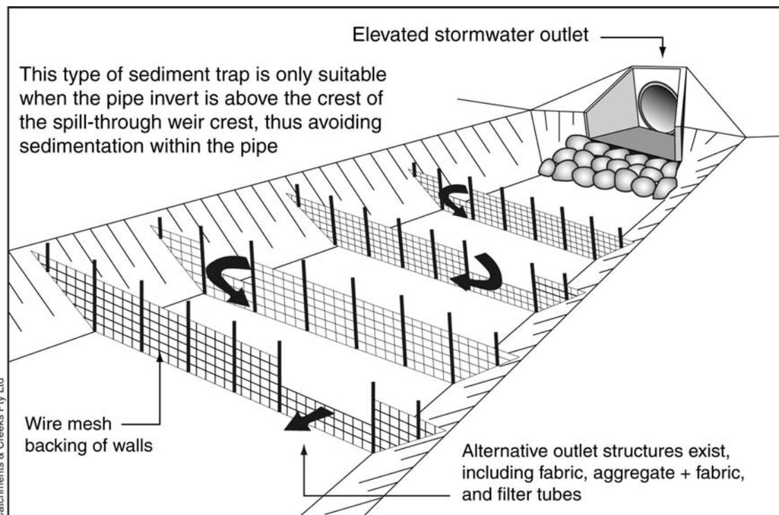
**Figure 2 – Partially enclosed coarse sediment trap located at a stormwater outlet**
