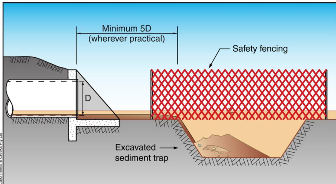
**Figure 1 – Recessed sediment trap suitable for pipe outlet with a pipe invert close to the elevation of the outlet channel**
