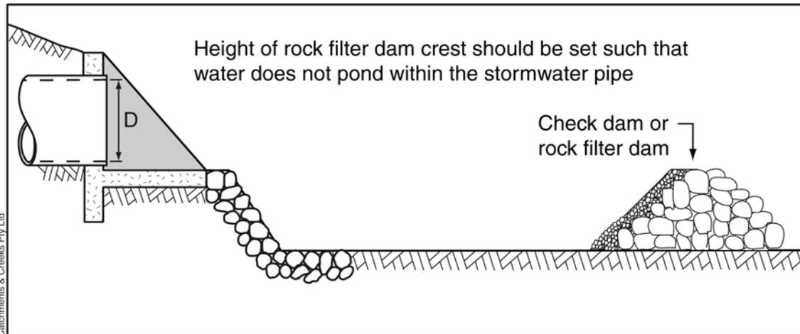
**Figure 5 – Rock filter dam placed downstream of an elevated stormwater outlet**
