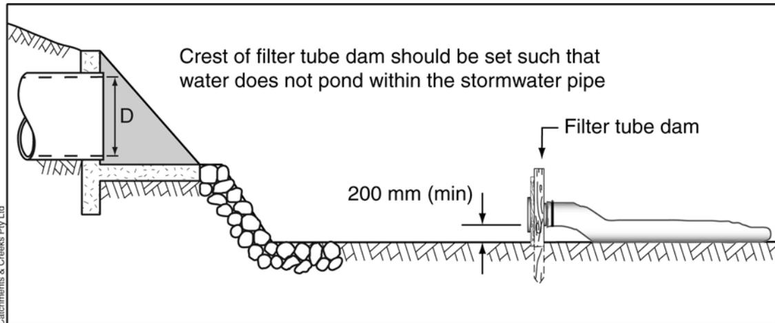
**Figure 4 – Filter tube dam placed downstream of an elevated stormwater outlet**
