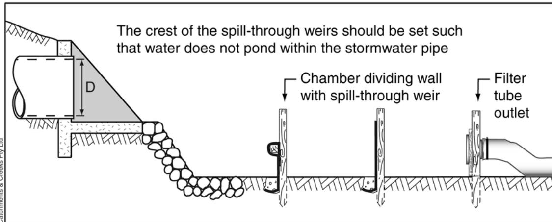
**Figure 3 – Coarse sediment trap placed downstream of an elevated stormwater outlet**
