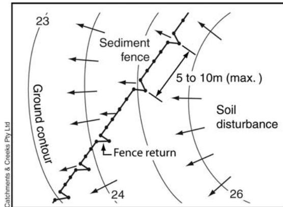
**Figure 2 – Fence install down a slope**
