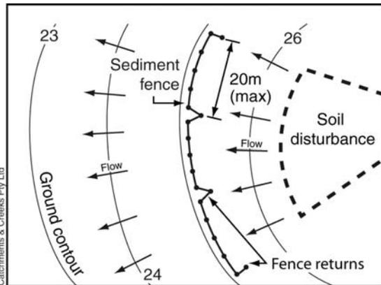
**Figure 1 – Fence installed along the contour**
