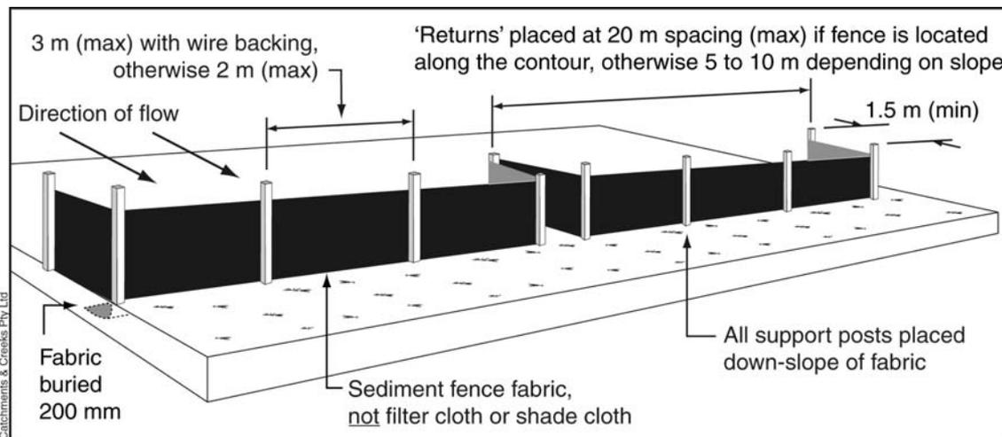
**Figure 5 – Typical installation of a sediment fence**
