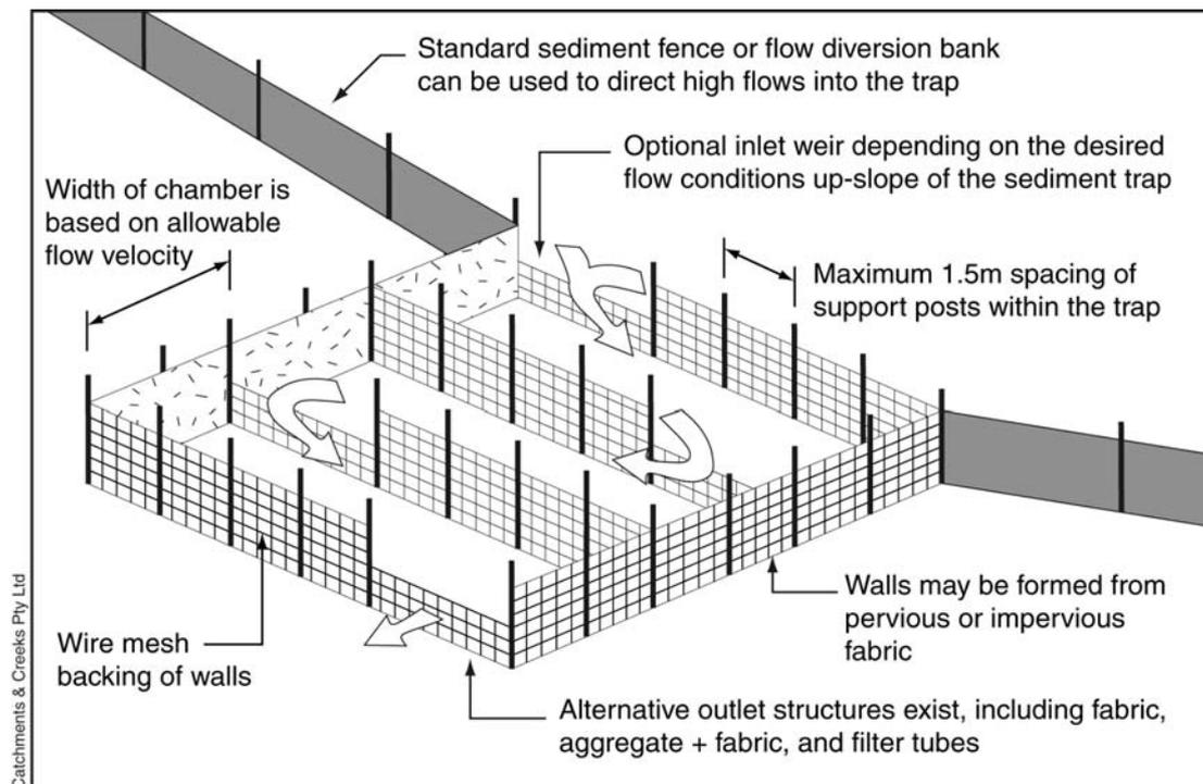
Figure 14 – Coarse sediment trap outlet structure
