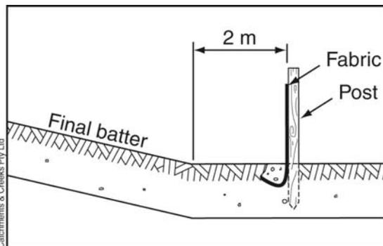
**Figure 3 – Fence installation at base of slope**
