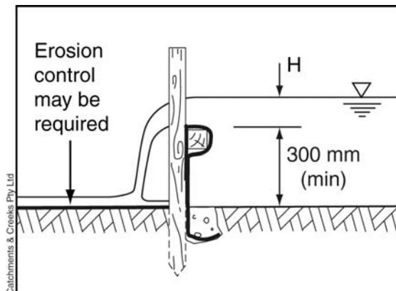
**Figure 13 – Side profile of a spill-through weir**
