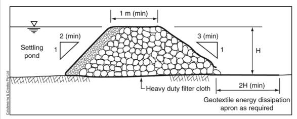
Figure 7 - Rock filter dam outlet system with aggregate and geotextile filter
