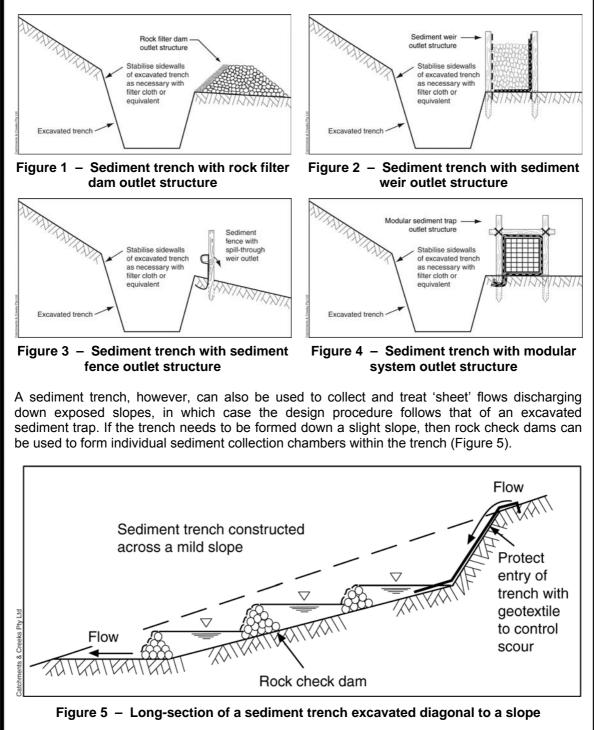
A rock filter dam outlet structure typically contains two different categories of rock, those being:
