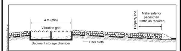
Figure 2 - Typical layout of vibration grid with rock ramps
