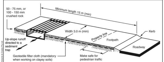
Figure 1 – Typical layout of vibration grid with rock ramps
