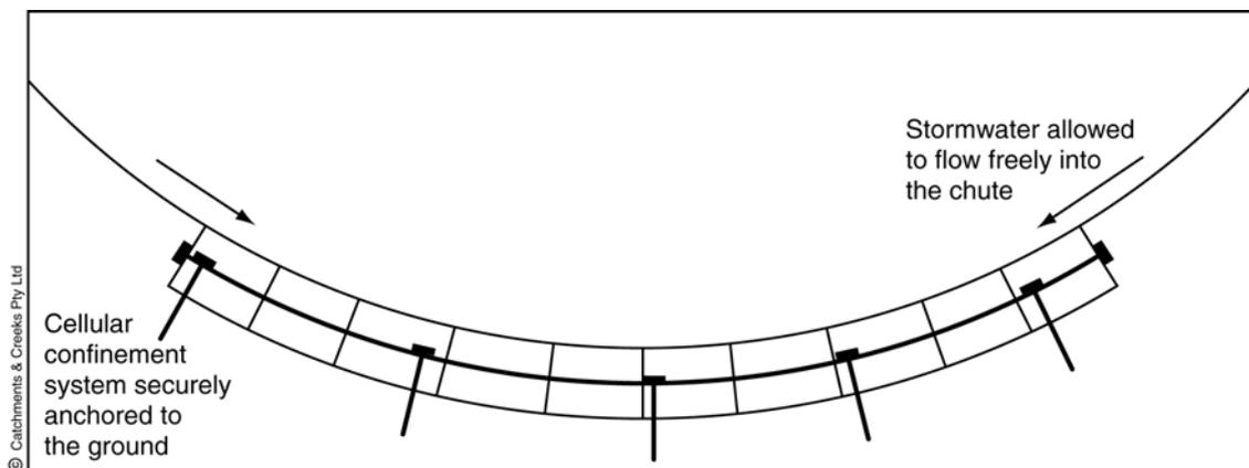
Figure 1 – Placement of cellular confinement system within a chute with concave profile
