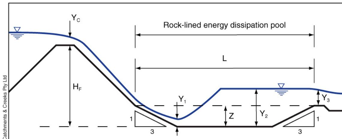
**Figure 2 – Typical profile of rock-lined energy dissipation pool**
