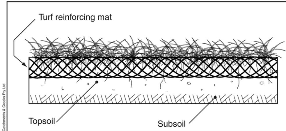
**Figure 1 – Diagrammatic representation of a three-dimensional turf reinforcement mat**
