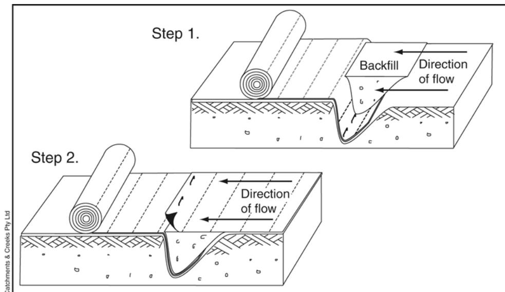
**Figure 2 – Anchoring of upstream edge of mat**
