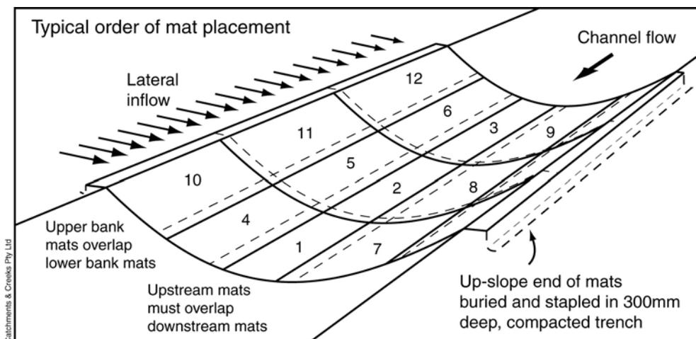
**Figure 3 – Placement of mats along channel which received lateral inflow**
