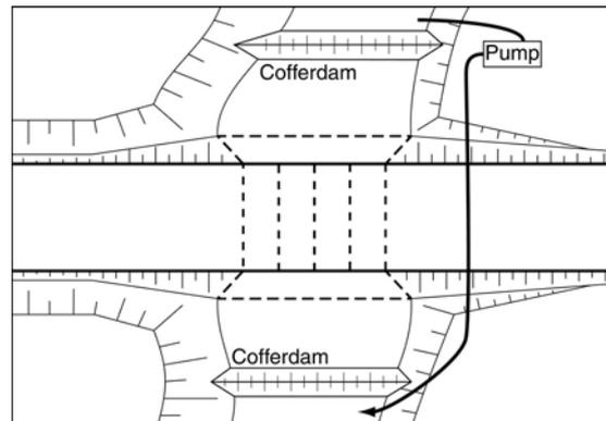
**Figure 2 – Cofferdam with pumped bypass flow**
