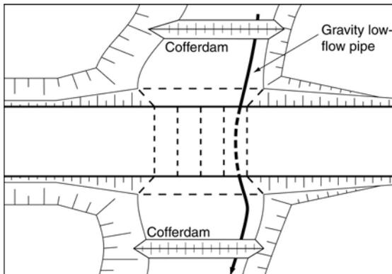
**Figure 1 – Cofferdam with gravity bypass pipe**
