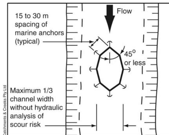
**Figure 3 – Installation of a silt curtain around a mid-channel disturbance**
