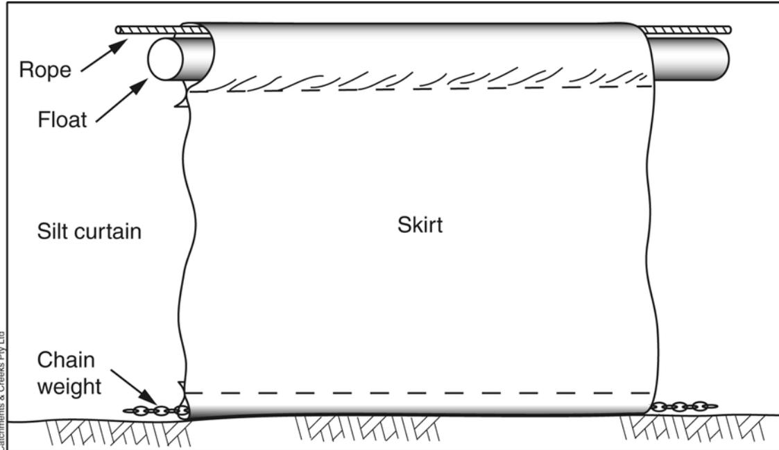
**Figure 1 – Typical features of a floating silt curtain**
