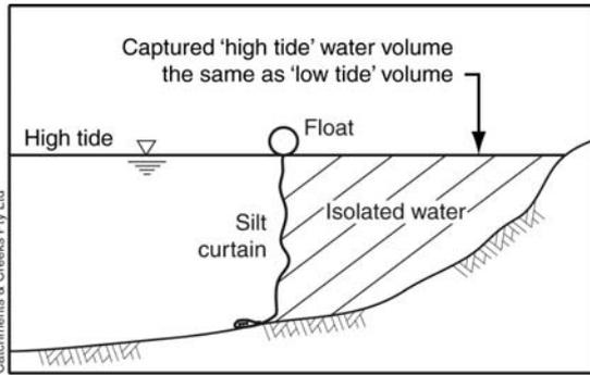
**Figure 7 – Near vertical curtain at high tide**
