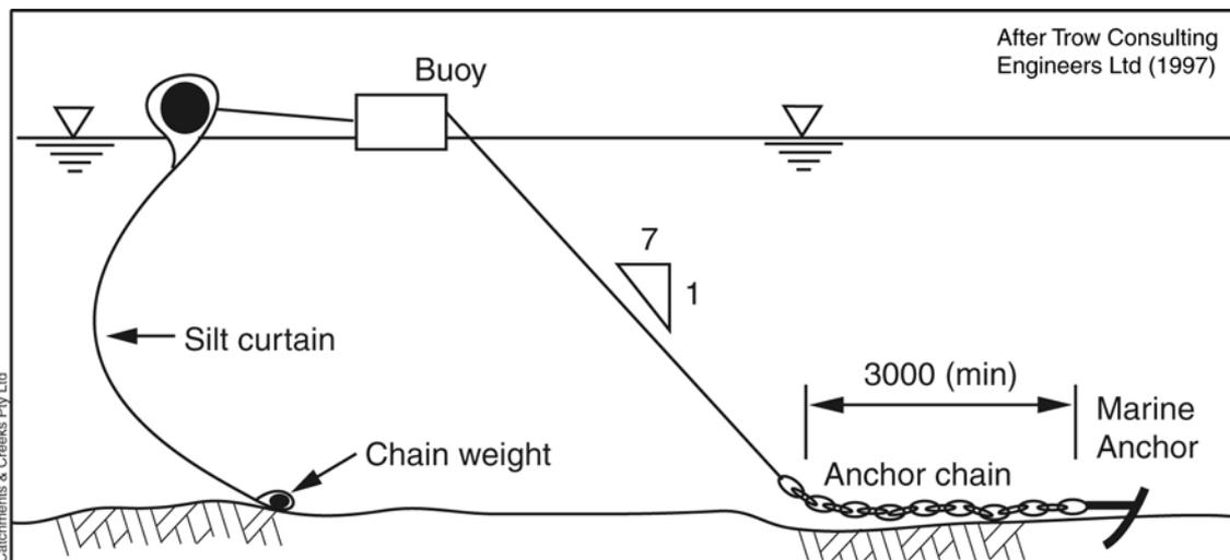
**Figure 5 – Typical marine anchorage system**
