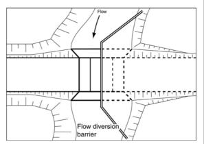
Figure 3 – Stage 1 of culvert construction using an isolation barrier
