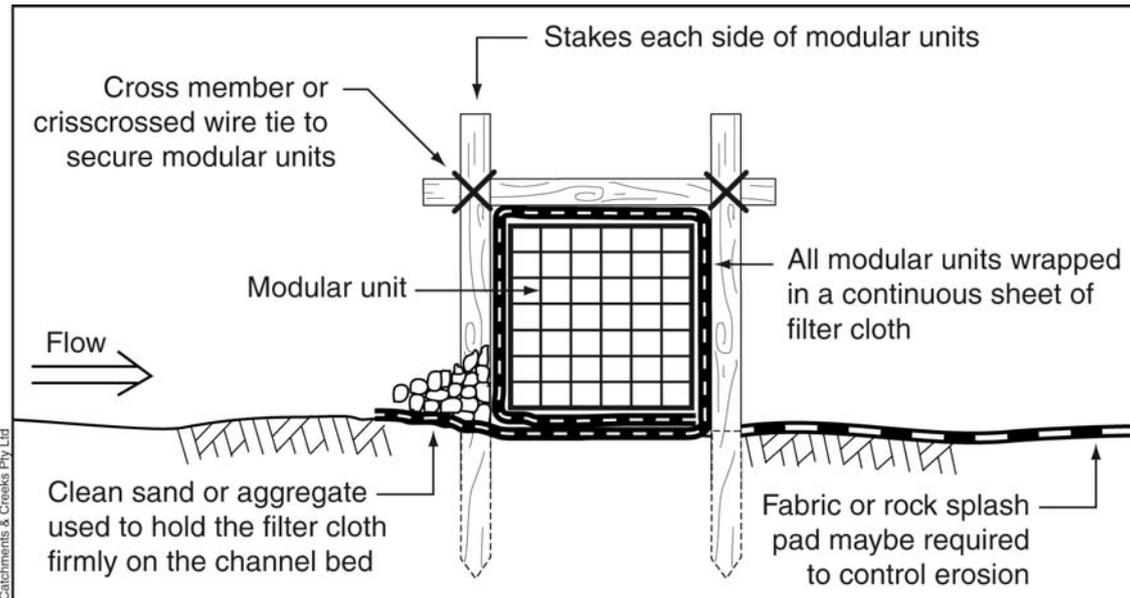
**Figure 3 – Typical installation of modular units on channel bed**
