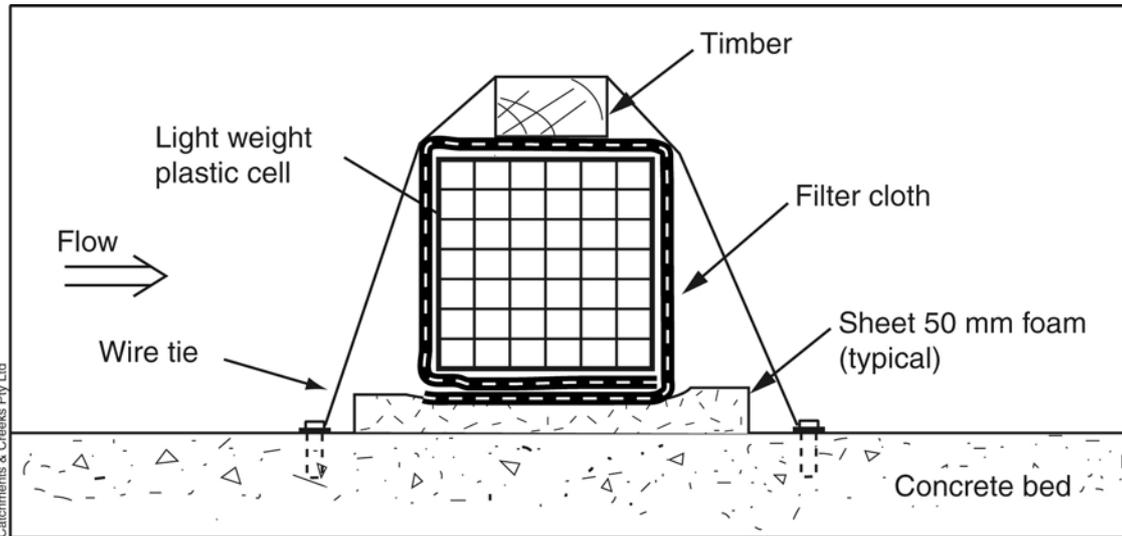
**Figure 5 – Typical installation of modular sediment barrier within a concrete drain**
