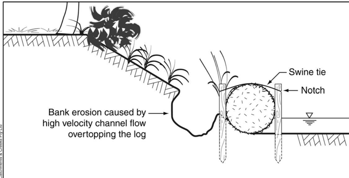
**Figure 4 – Example of potential bank erosion caused by high velocity channel flow overtopping the logs before bank vegetation is full established**
