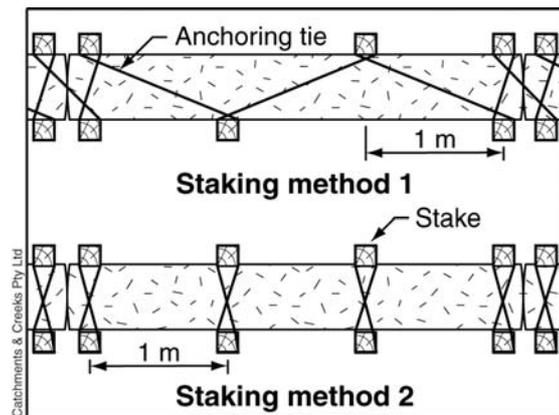
Figure 3 – Various methods of stake placement
