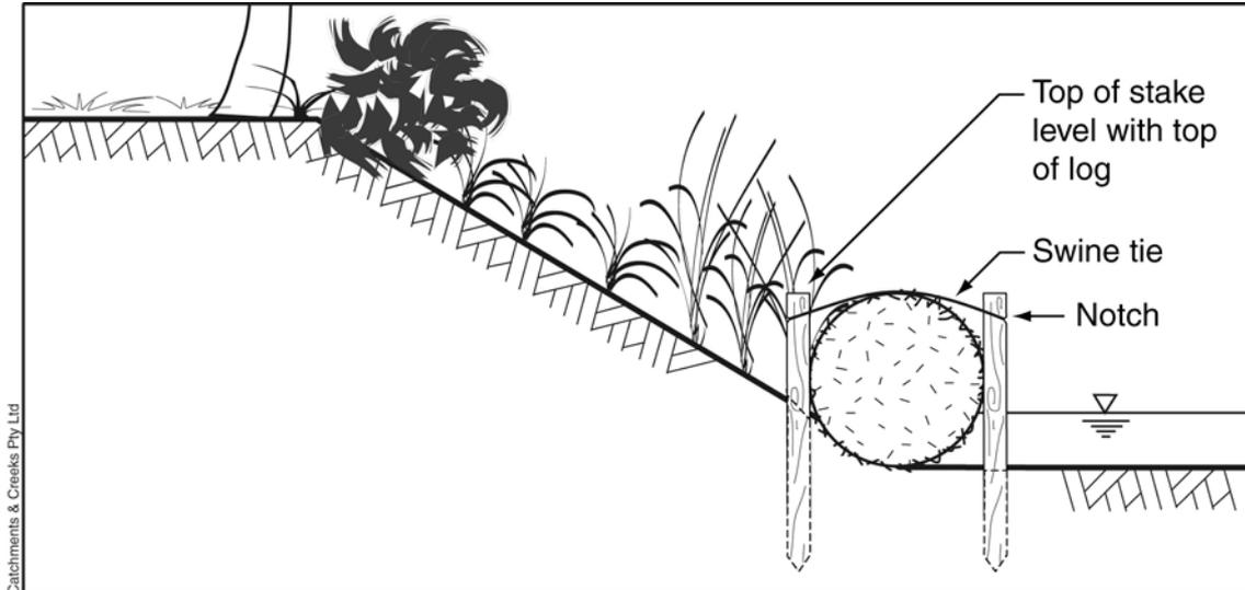
Figure 1 – Typical placement of geo log at toe of stream bank
