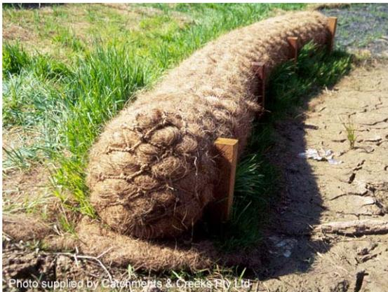
**Photo 1 – Geo log (log is being displaced at an industry field day, not on an active erosion site)**
