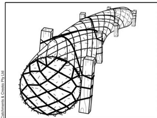
Figure 2 – Typical anchorage of geo log
