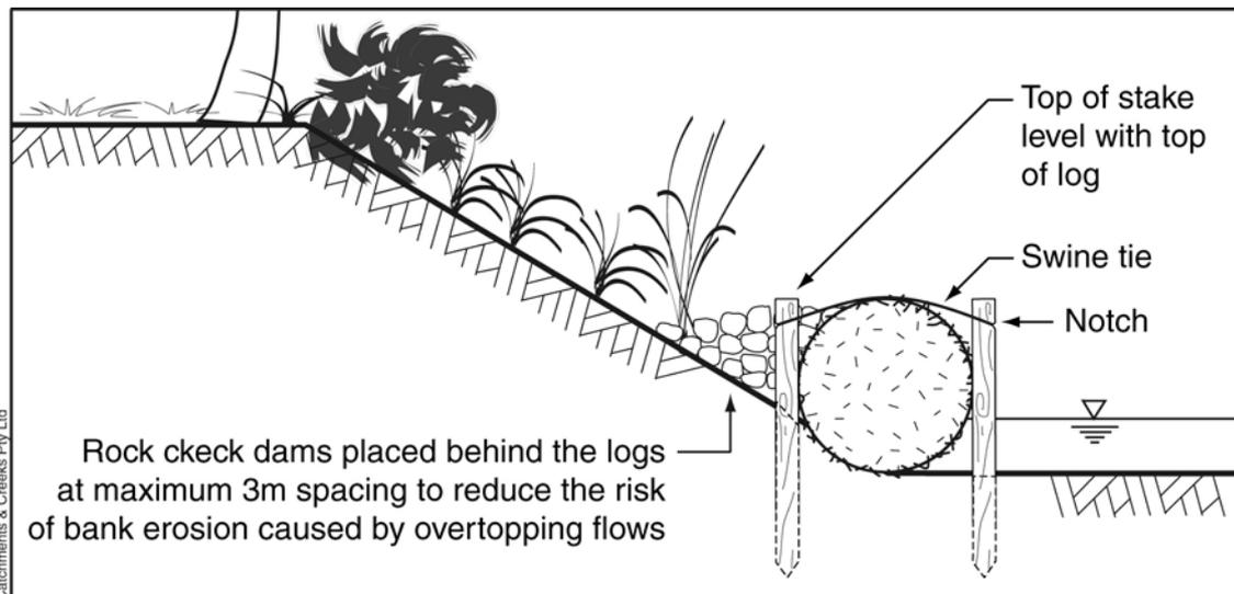
**Figure 5 – Optional placement of rock check dams to reduce the risk of bank erosion behind the logs caused by overtopping stream flows**
