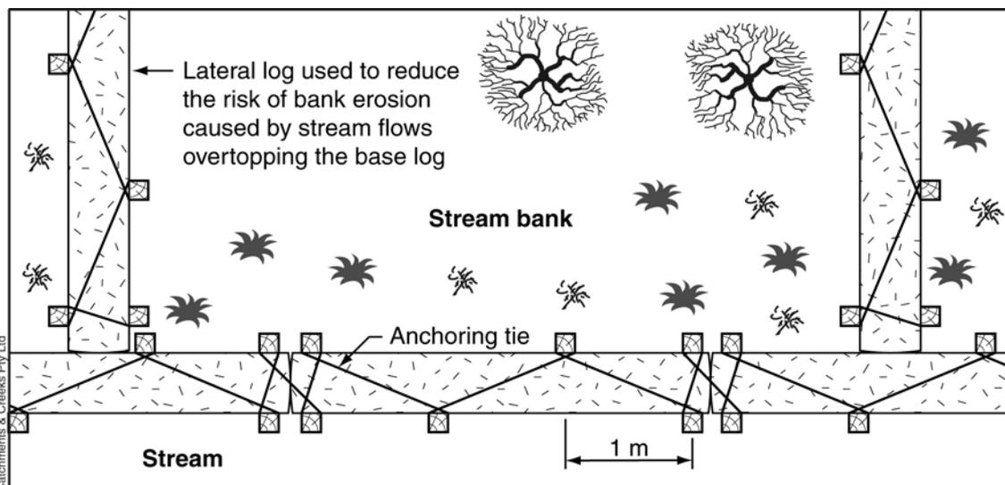
**Figure 6 – Optional placement of lateral logs to reduce the risk of bank erosion**
