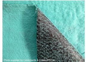
Photo 4 – Composite fabric with the woven (black) backing being the down-slope face of the sediment fence In 'dry' streams during periods when:
