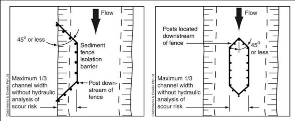
Figure 1 – Isolation of bank disturbance
