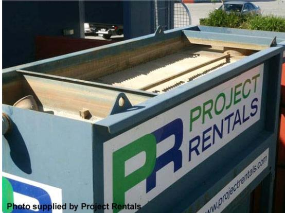
Portable settling (lamella) tank
