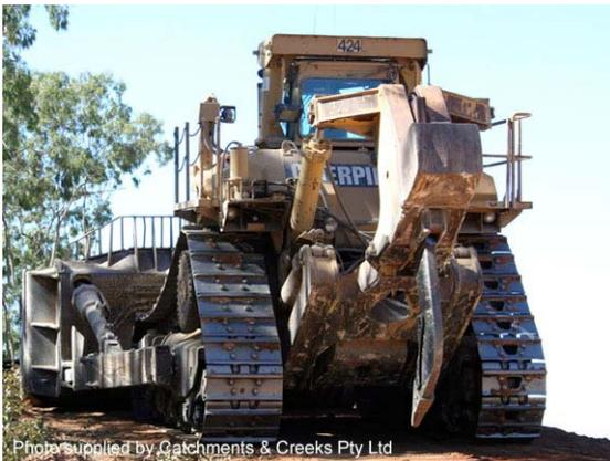
**Photo 3 – Crawler dozer with ripper (rear attachment)**
