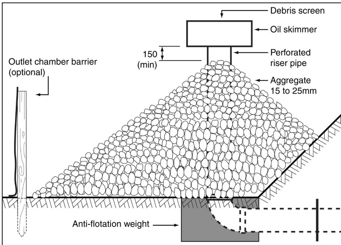
**Figure B31 – Typical details of riser pipe outlet with aggregate filter**
