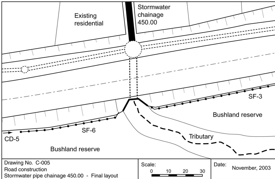
**Figure D14 – Final road layout at chainage 450.00 (Dwg C-005)**
