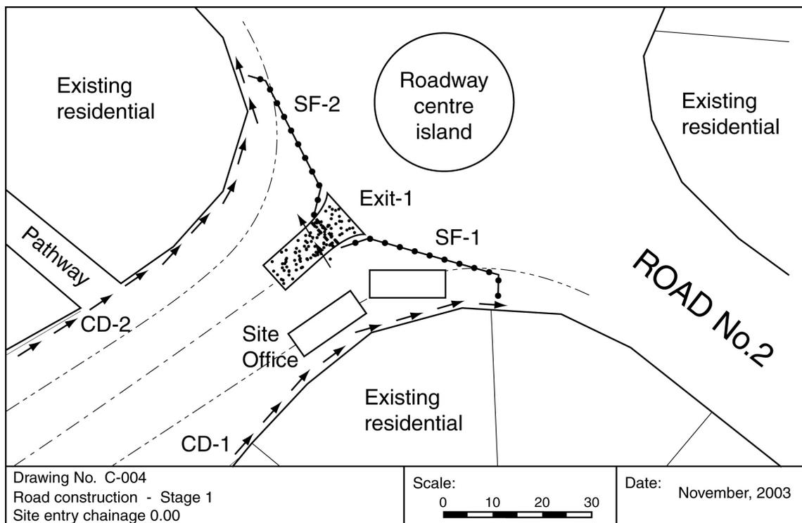
Figure D13 – Details of road intersection (Dwg C-004)
