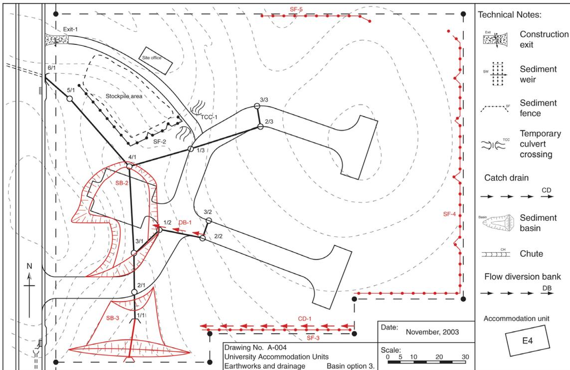
Figure D6 – Option 3 for establishment of a Sediment Basin
