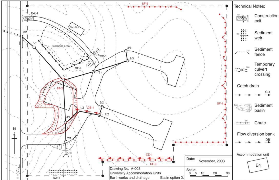
Figure D5 – Option 2 for establishment of a Sediment Basin
