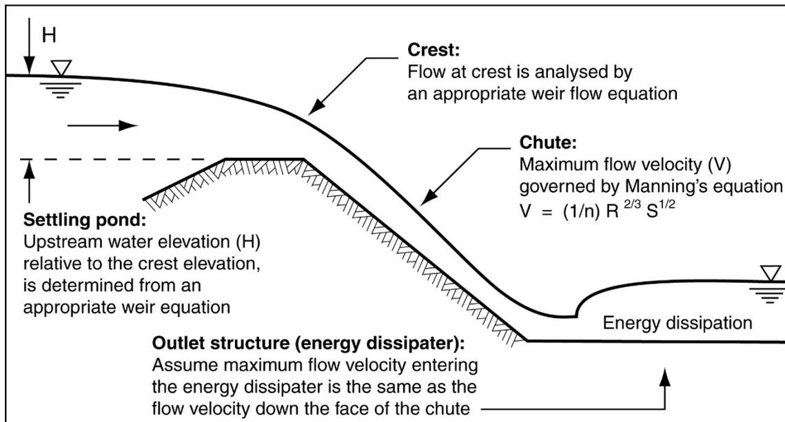
**Figure B36 – Hydraulics of sediment basin spillways**
