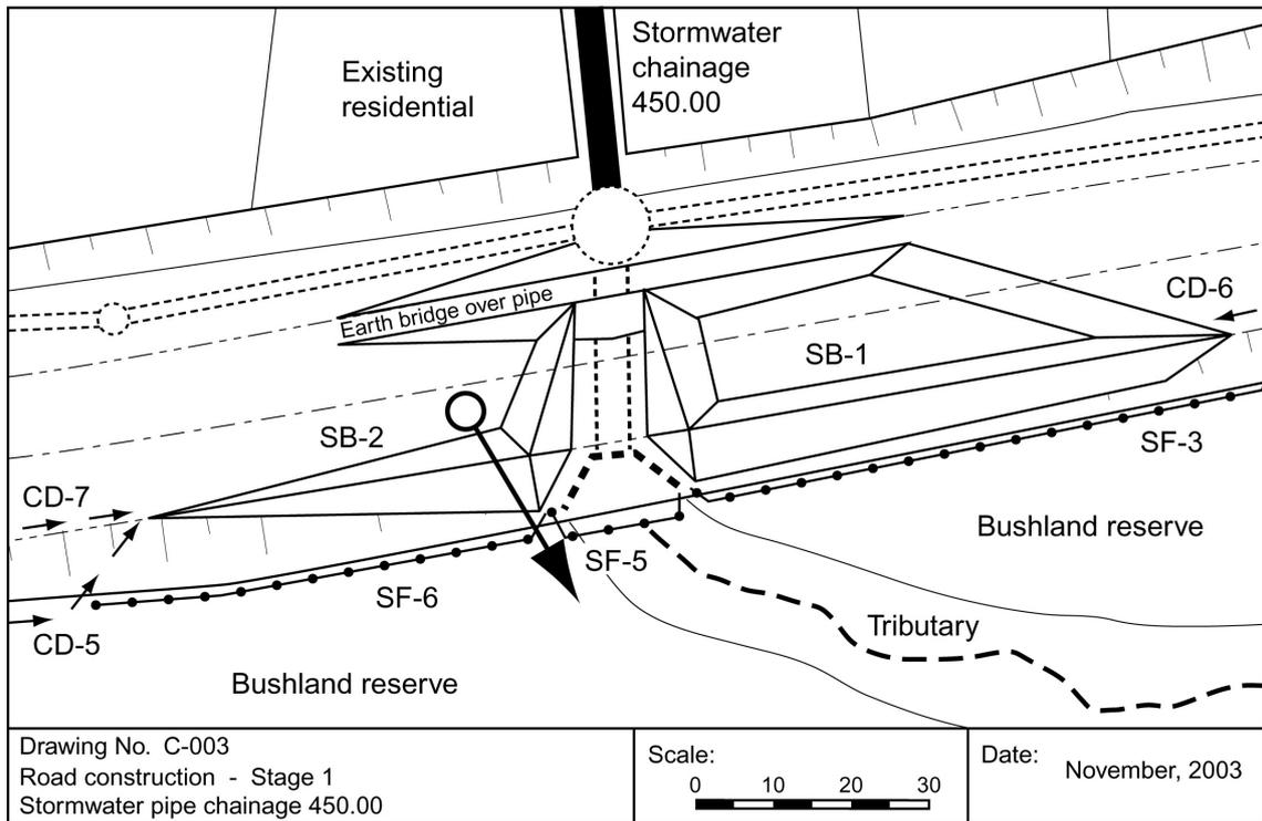
Figure D12 – Details of sediment basins (Dwg C-003)
