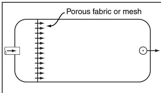
Figure B24(a) – Porous barrier inlet chamber
