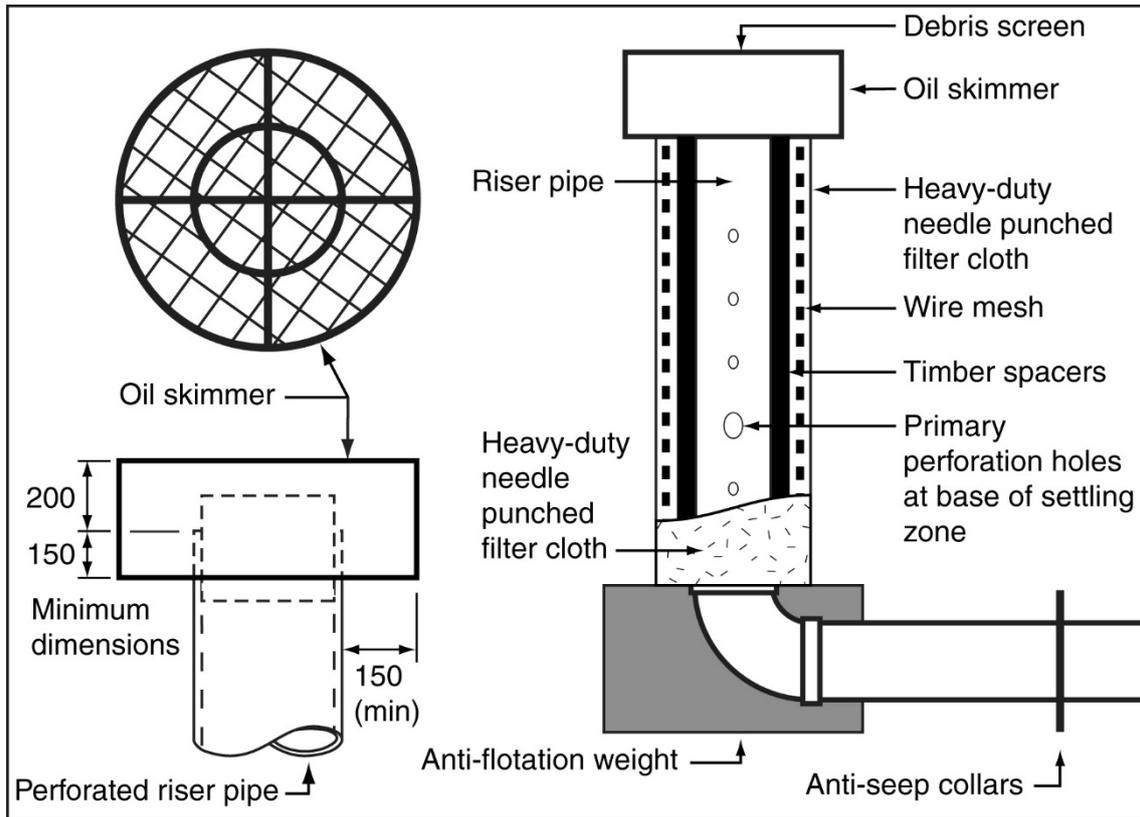
**Figure B30 – Typical details of riser pipe outlet with fabric filter**
