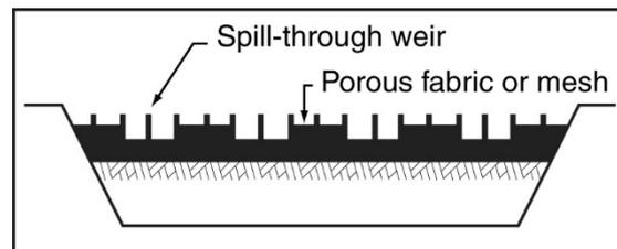
**Figure B27(b) – Barrier with multiple spill-through weirs**
