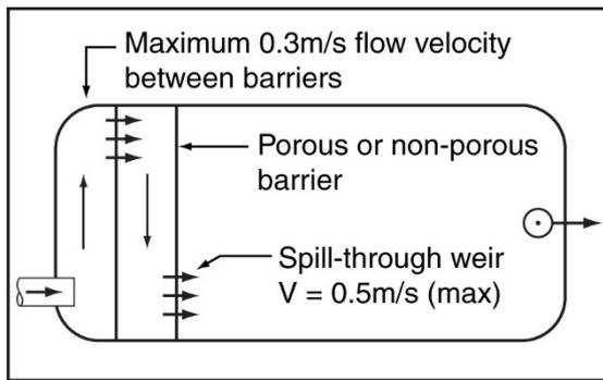
**Figure B26(a) – Alternative inlet chamber design**
