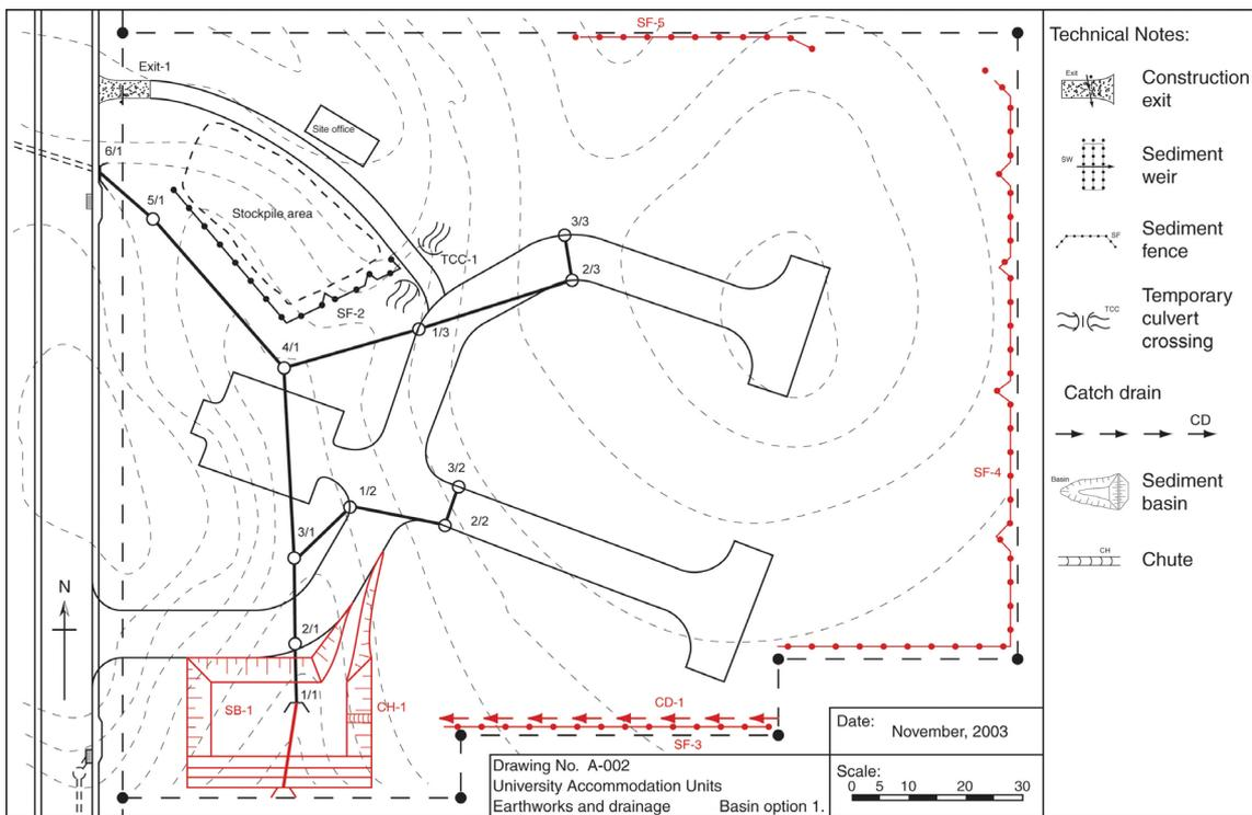
Figure D4 – Option 1 for establishment of a *Sediment Basin*
