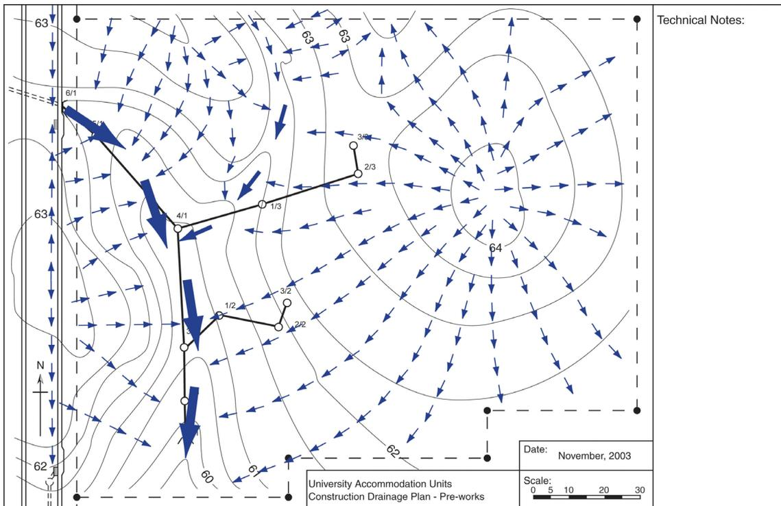
Figure D2 – Site drainage prior to development
