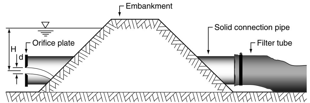
**(d) Filter tube low-flow outlet with orifice plate**
