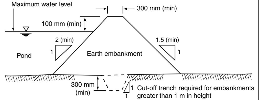
**(b) Typical profile of earth embankment**
