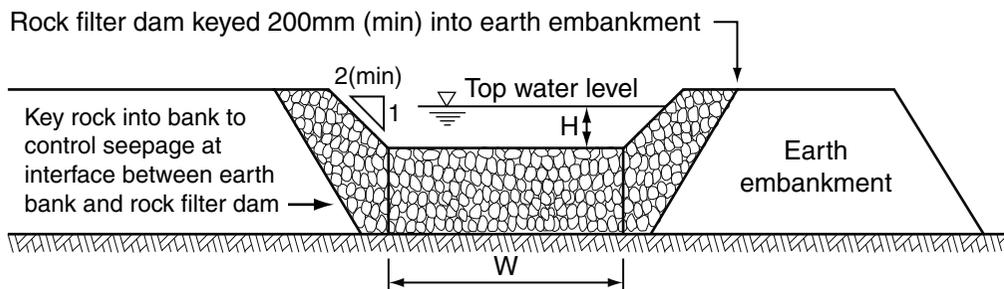
**(e) Rock filter dam with overflow spillway**
