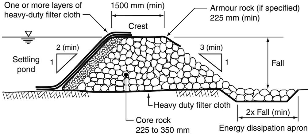
**(c) Rock filter dam low-flow outlet with geotextile filter**
