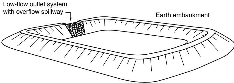
**(a) Settling pond with rock filter dam low-flow outlet**
