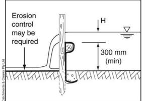
Figure 13 – Side profile of a spill-through weir
