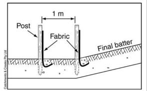
Figure 4 – Double sediment fence installed at the based of a fill slope
