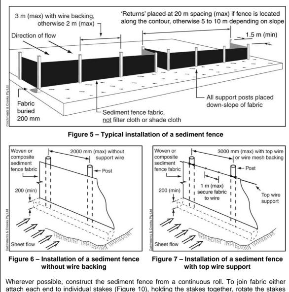
Wherever possible, construct the sediment fence from a continuous roll. To join fabric either attach each end to individual stakes (Figure 10), holding the stakes together, rotate the stakes 180 degrees, then drive the two stakes into the ground; or overlap the fabric to the next support post (Figure 11).
