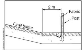
Figure 3 – Fence installation at base of slope
