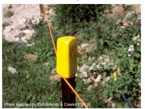
Photo 28 – Safety cap on a steel stake
