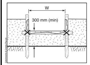
Figure 12 – Spill-through weir profile
