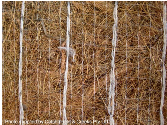
Photo 9 – Synthetic mulch anchorage
