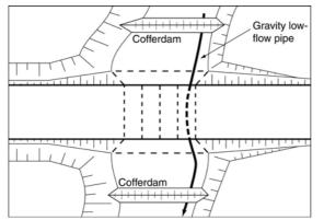
Figure 1 – Cofferdam with gravity bypass pipe
