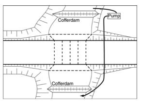
Figure 2 – Cofferdam with pumped bypass flow
