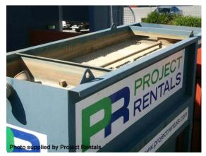
Portable settling (lamella) tank
