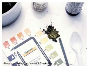
Field testing of soil pH
