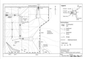
Erosion and sediment control plan
