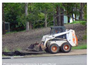
Photo 11 – Skid-steer loader ("bobcat" is a commercial brand name)
