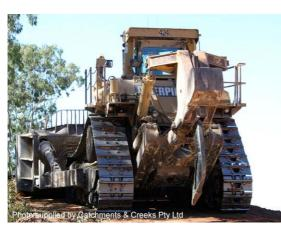
Photo 3 – Crawler dozer with ripper (rear attachment)
