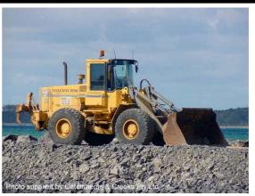
Photo 8 – Loader (wheel loader), crawler loaders are also available
