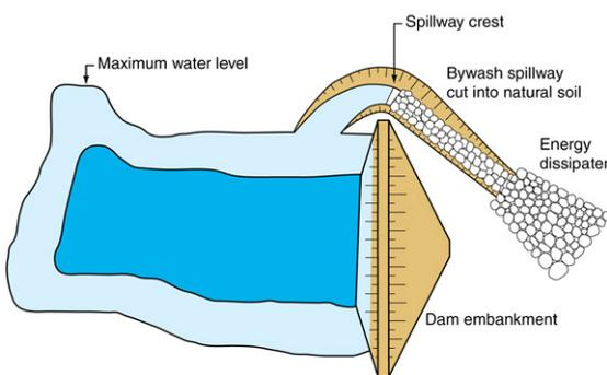
Figure 22 – Spillway cut into virgin soil
