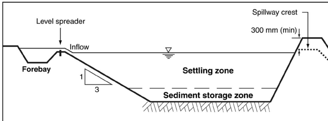
Figure 2 – Long-section of a typical Type B basin
