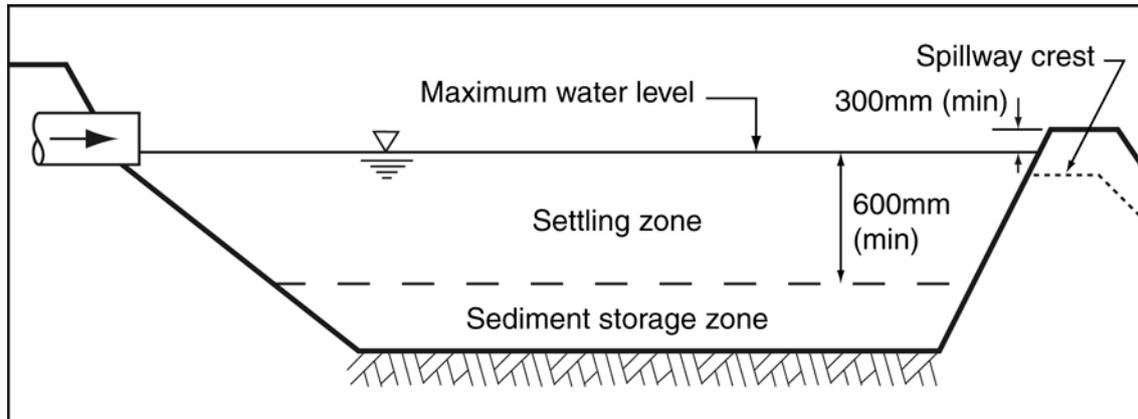
**Figure 4 – Settling zone and sediment storage zone**
