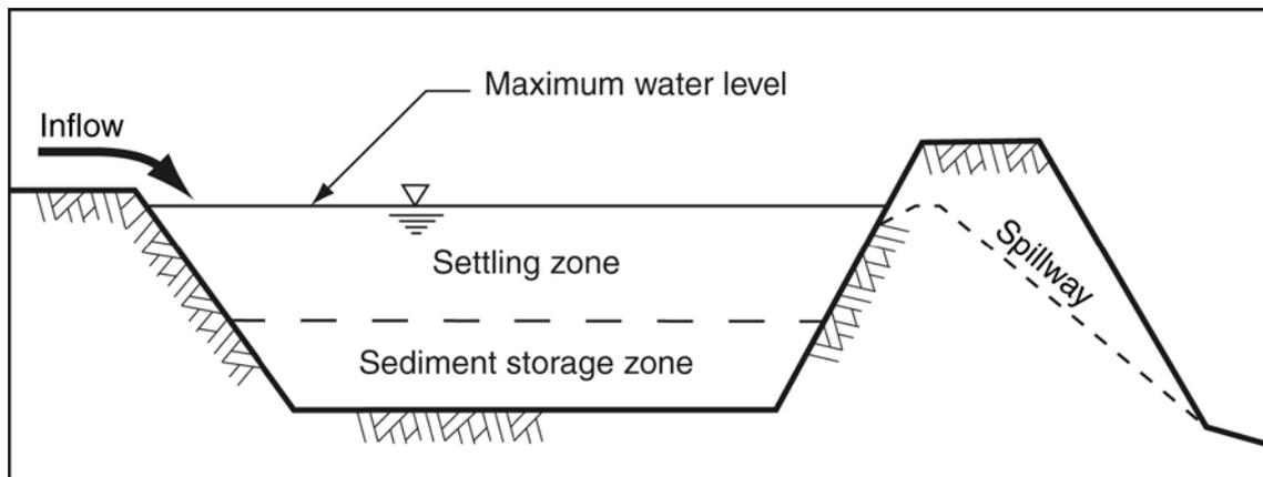
Figure 5 – Settling zone and sediment storage zone
