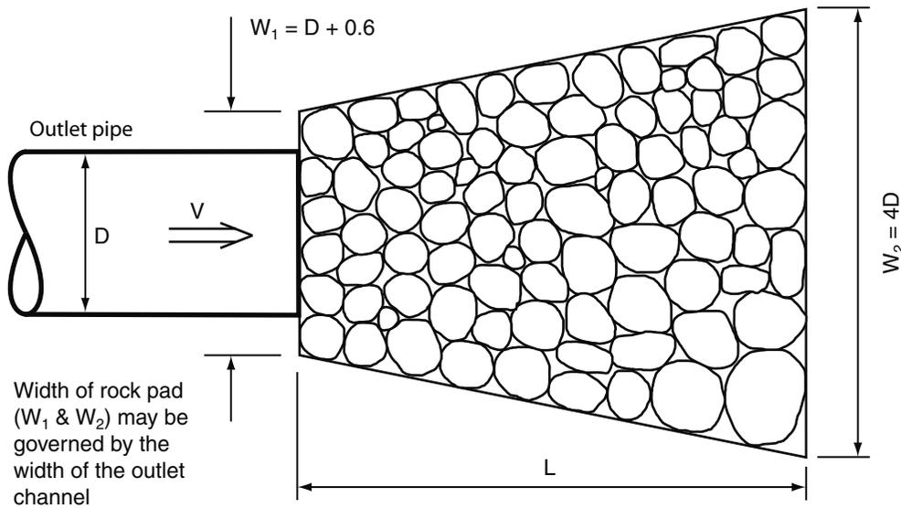
(a) Typical layout of a rock pad outlet structure for a pipe outlet
